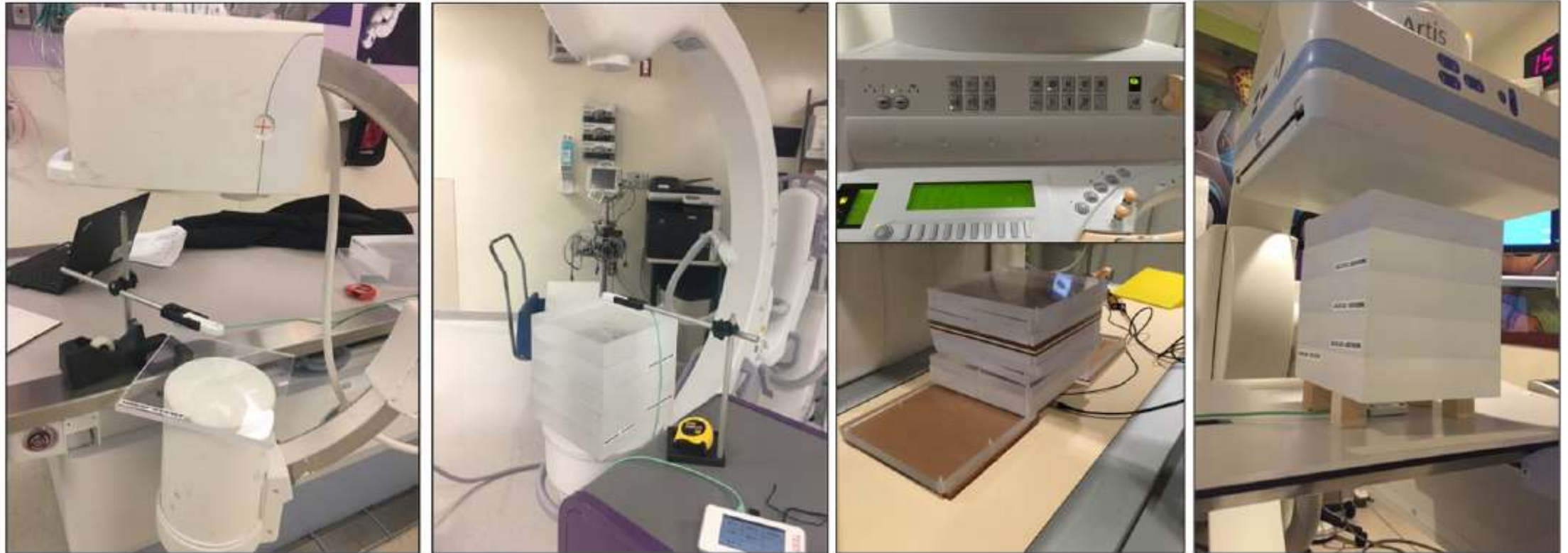
Figure 1. Measurement geometry and general equipment setup for (a) mini C-arms, (b) mobile C-arms (slabs of PMMA placed directly on the input II or FPD), (c) general fluoroscopes (GF), (d) interventional angiographic radiology (IRR), interventional cardiac (IRC), and electrophysiology (EP) equipment.
